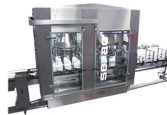
RB Atex/Ex-proof: Filler-Capper for flammable liquids
