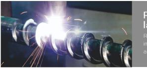
PTA bimetallic spraying, laser dissolution spraying
