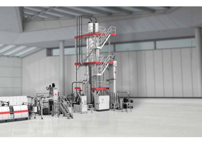
**Solid state polycondensation** – optionally for the **IV increase of PET and outstanding decontamination**. The regranulate after the Starlinger iV+ process is suitable for **food contact applications** such as bottle-tobottle or bottle-to-sheet. The process has achieved several national and brand-owner approvals.
