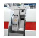
The high-vacuum degassing extruder reduces viscosity loss during extrusion and purifies the melt from volatile contamination. The waterfree vacuum pump reduces production and maintenance costs.
