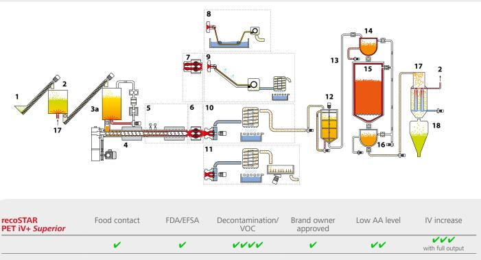
The combined decontamination steps – first the flakes in the vacuum dryer upstream of the extruder (FG+), then the pellets in the SSP reactor downstream of the extruder (iV+) – result in the highest possible pellet quality. This superior decontamination reduces AA and VOC to a minimum. Optionally, the two steps can be separated to double the capacity: Food-contact flakes and/or food-contact pellets can be produced.
