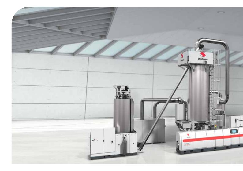
**State-of-the-art recycling** technology for the in-house recycling of PET flakes from bottles, preforms, strapping bands and sheets as well as for the **recycling of post-consumer bottle flakes** after the washing process. The **end product is melt-filtrated**, **uniform granulate** that can be used for a wide range of applications.
